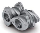
Alternating channel depth and tip clearance with each revolution, same as T6 screw element Geometrically self-cleaning, with asymmetric profile | Elimination of pressure/shear peaks associated with standard kneading elements
