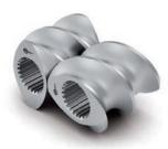
Screw elements for feeding solids, melt or viscous medium with single, double and triple flight design. Tightly intermeshing profile with Erdmenger design and therefore self-cleaning screws. CPM Extrusion Group is the supplier of more than 30 OEM brands ranging from 10mm through 410 mm.
